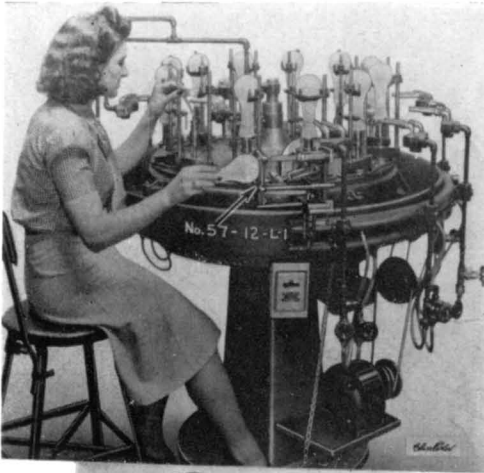
The Eisler 12-position automatic bulb-sealing machine, 1935, making hand-pulling (as illustrated below ) no longer necessary.
